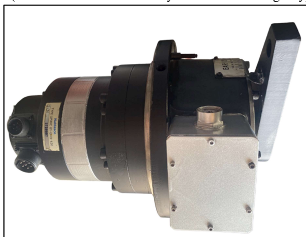
(An actuator reconditioned by an unauthorized agency)
